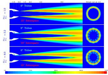
Turbulent Kinetic Energy  $[k]=m^2/s^2$ - NPR <br/>  $(p_{0,n}/p_\infty)=$  4.0 - Nozzle $60^\circ$  Upstream Injection
