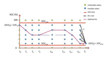
Calculation of the optimal state-of-charge profile for a model based upon the Ohio State Challenge X vehicle shown above.
