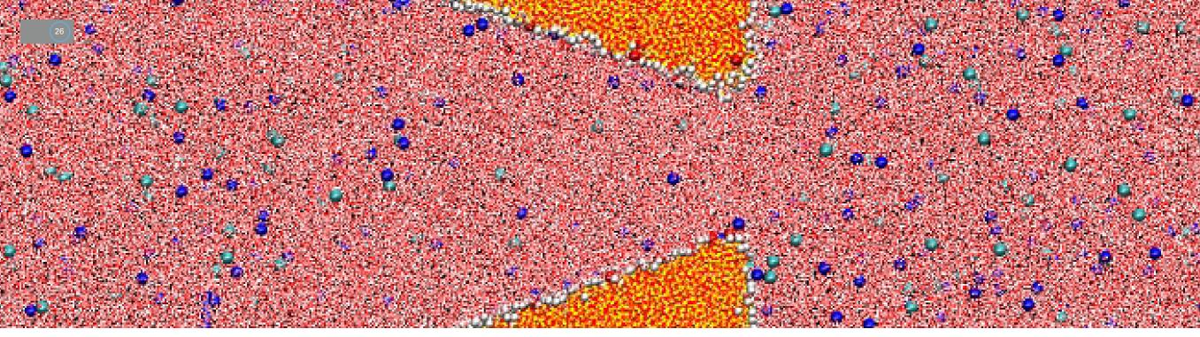
Fully atomistic simulations of electroosmotic flow in a "nano-nozzle" device.
