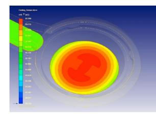
Three-dimensional simulation of an injection-molded lens, showing cooling temperature gradients.
