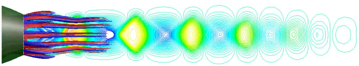
A qualitative image of the supersonic flow field exhausting the convergent-divergent nozzle with fluidics on.
