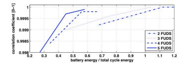
Linear correlation with respect to battery capacity: As the battery size of a PHEV increases, the optimal state-of-charge profile shows a higher correlation coefficient to a linear fit.
