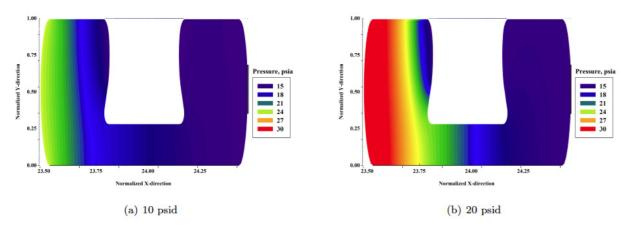
(Right) An analysis of air leakage of main interface seals – shown here as an orange ring – used in NASA's International Low Impact Docking System (iLIDS). (above) Characterization of computational pressure profiles of a potential main interface seal for docking at the International Space Station and other new spacecraft.
