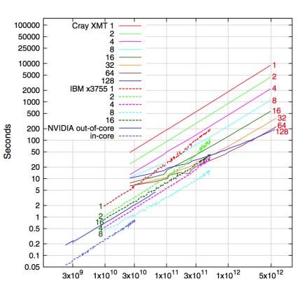
Comparison of performance measures of parallel supercomputers that employ various architectures: (1) Cray XMT, 128 proc, 500 MHz, 1-TB; (2) IBM x3755, 2.4-GHz Opterons, 16-core, 64-GB; (3) NVIDIA FX 5800 GPU, 1.296 GHz, 240 cores, 4-GB device memory.
