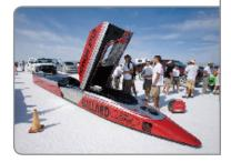
BuckeyeBullet2, the world's first land-speedrace research vehicle powered by hydrogen fuelcells, is designed and built by students at The Ohio State University's Center for Automotive Research.
