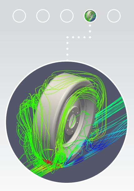
Using Ohio Supercomputer Center systems, Ohio State's Cary Bork simulates airflow within the wheel well of the Buckeye Bullet land speed racer with the vehicle traveling at 300 mph.
