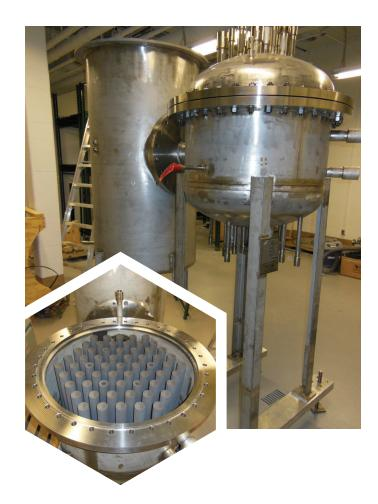
are currently testing the two modes of air ingress to determine under which conditions each could dominate. This information will be used to improve VHTR prototype designs and accident mitigation. Generation IV designs will maintain today's high level of safety while shifting from the current paradigm of mastering accidents to excluding accidents entirely. •
