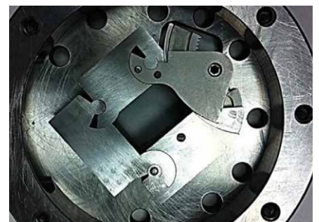
{LEFT} The design algorithms help synthesize the mechanism inside a variable geometry extrusion die. The die extrudes plastic parts with varying cross-section, a novel capacity in extrusion. {CENTER} Model of the design in the above figure. {RIGHT} The mechanism is inside the die shown. The variation in the extrusion as it exits the die is seen here.
