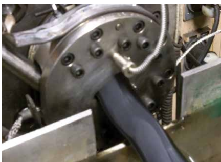
{LEFT} The design algorithms help synthesize the mechanism inside a variable geometry extrusion die. The die extrudes plastic parts with varying cross-section, a novel capacity in extrusion. {CENTER} Model of the design in the above figure. {RIGHT} The mechanism is inside the die shown. The variation in the extrusion as it exits the die is seen here.
