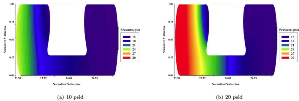
(Right) An analysis of air leakage of main interface seals – shown here as an orange ring – used in NASA’s International Low Impact Docking System (iLIDS). (above) Characterization of computational pressure profiles of a potential main interface seal for docking at the International Space Station and other new spacecraft.
