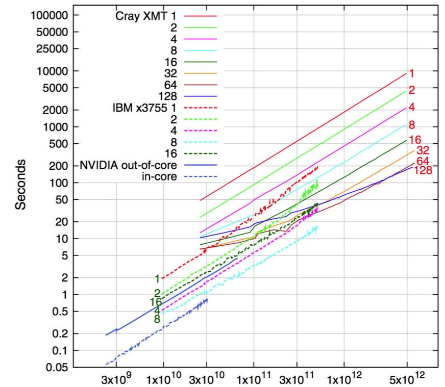
*Comparison of performance measures of parallel supercomputers that employ various architectures: (1) Cray XMT, 128 proc, 500 MHz, 1-TB; (2) IBM x3755, 2.4-GHz Opteron, 16-core, 64-GB; (3) NVIDIA FX 5800 GPU, 1.296 GHz, 240 cores, 4-GB device memory.*
