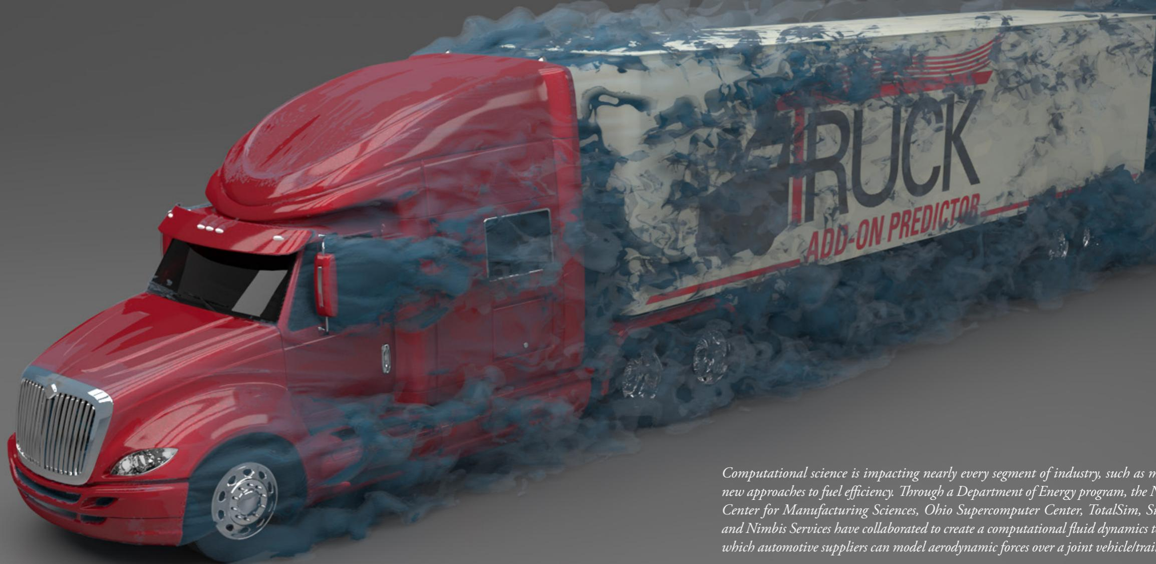
*Computational science is impacting nearly every segment of industry, such as modeling new approaches to fuel efficiency. Through a Department of Energy program, the National Center for Manufacturing Sciences, Ohio Supercomputer Center, TotalSim, SimaFore and Nimbis Services have collaborated to create a computational fluid dynamics tool with which automotive suppliers can model aerodynamic forces over a joint vehicle/trailer body.*
