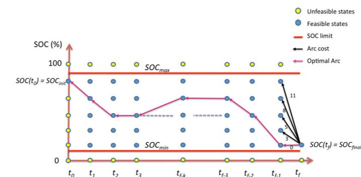
*Calculation of the optimal state-of-charge profile for a model based upon the Ohio State Challenge X vehicle shown above.*
