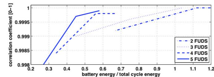
*Linear correlation with respect to battery capacity: As the battery size of a PHEV increases, the optimal state-of-charge profile shows a higher correlation coefficient to a linear fit.*
