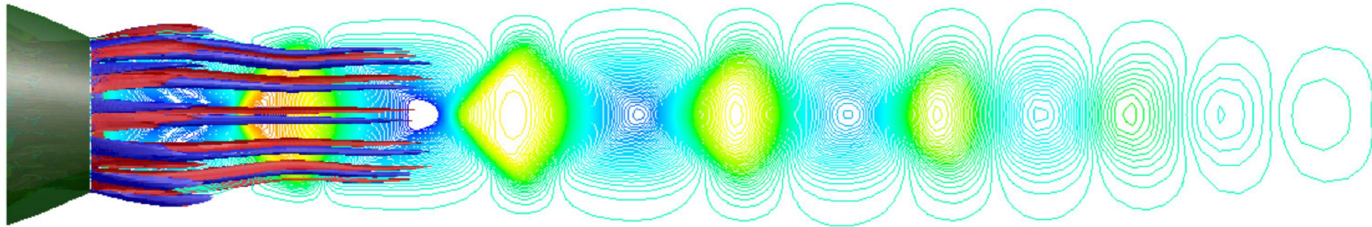
A qualitative image of the supersonic flow field exhausting the convergent-divergent nozzle with fluidics on.
