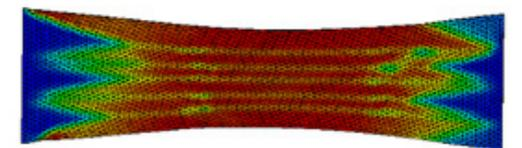
*(above) When a sample with uniform microstructure is stretched laterally, the microstructure evolves to form a pattern of stripes, giving rise to a remarkably soft elastic response.*
