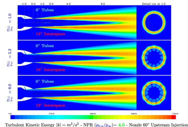
The effect of injection on the turbulent kinetic energy levels for an upstream injection (near-by the nozzle throat) at 60 degrees angle.
