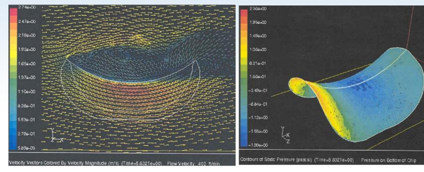
High Speed Conveying Create Vortices Shedding... ...'Rocking Chips' NOT GOOD!
